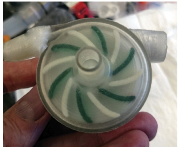
FIGURE E5. A close-up picture of the turbine impeller and shroud of the iATVA prototype 3 is presented. Six additional blades are produced separately using a high-accuracy 3-D micro stereolithography printer (Projet 1200; 3D Systems, Rock Hill, SC) from VisiJet FTX Green resin (3D Systems) and glued to the prototype 1 impeller. A total of 3 iATVA prototypes are tested in static as well as dynamic conditions.
