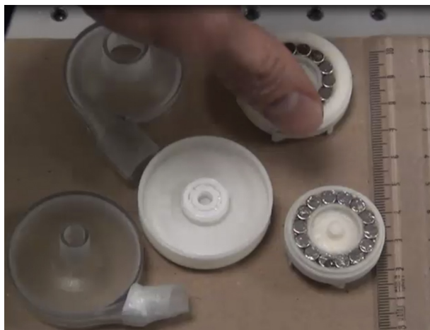
VIDEO 1. Assembly process of a magnetically coupled integrated aortic-turbine venous assist device (iATVA) with ceramic bearings. The iATVA prototype supporting a single-ventricle circulation, in vitro demonstrated through an instrumented mock-up flow loop. Video available at: http://www.jtcvsonline.org/article/S0022-5223(18)30717-7/fulltext .
