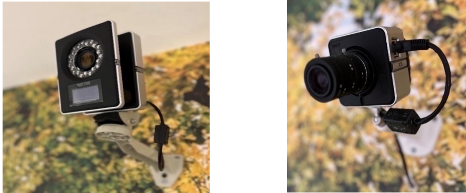
Picture 5. Infrared cameras and HD cameras of the gait analysis system
