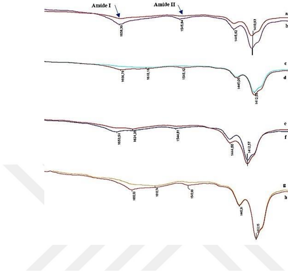
Figure 47. Peptide self-assembly on catheter at 37°C FT-IR results a) NET1 washed b) NET1 c) NET2 washed d) NET2 e) NET3 washed f) NET3 g) NET4 washed h) NET4
