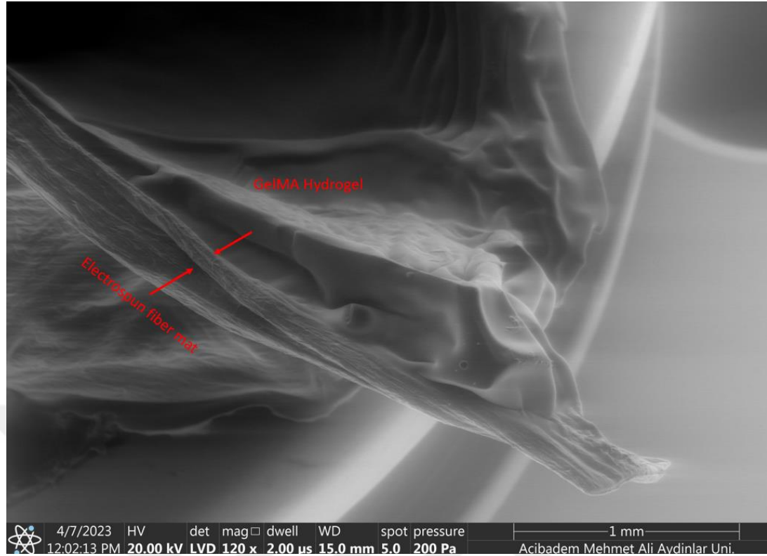
Figure 25 SEM image of the two layers of the tubular structure under low vacuum. Magnification: x120, Scale bar: 1 mm.
