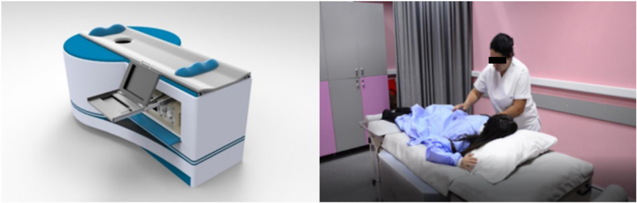
Figure 1. SAFE (Scan and Find Early) Microwave Imaging Device for breast cancer early screening and diagnostic: (a) SAFE industrial design, (b) SAFE's patient scanning process.
