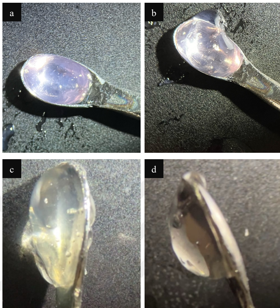
Figure 24. Stereomicrographs of hydrogels in spatula prepared with (a) 0.5% HA-1.5% Col HA-Col (1:1), (b) 0.66% HA- 1% Col solutions, and 0.66% HA- 1% Col hydrogel prepared with thiol-modified hyaluronan using PEGDA ratios of (c) 8:1 and (d) (2:1).
