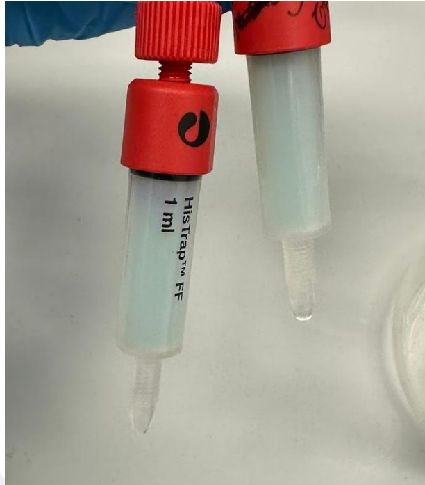
Figure 14: His-tag affinity columns during purification procedure.
