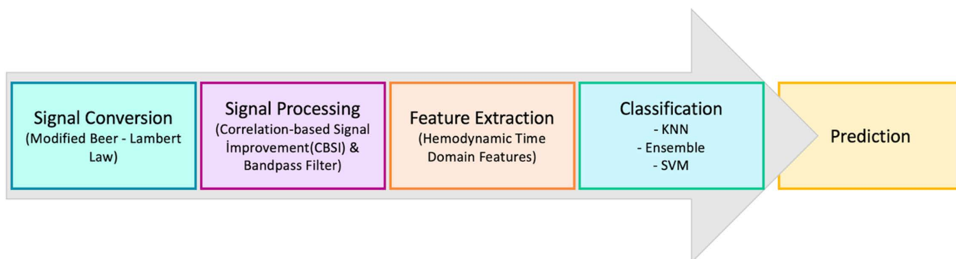
Fig 3. Overview of the Data Analysis Pipeline. The pipeline consists of four main stages: (1) Conversion of raw optical signals into relative changes in HbO concentration using Modified Beer-Lambert Law; (2) Preprocessing of HbO signals through Correlation-Based Signal Improvement (CBSI) and a Butterworth bandpass filter; (3) Feature Extraction, where hemodynamic time-domain features are extracted (e.g. mean, variance, kurtosis...); and (4) Classification through machine learning algorithms which include k-Nearest Neighbors (KNN), Ensemble, and Support Vector Machine (SVM).
